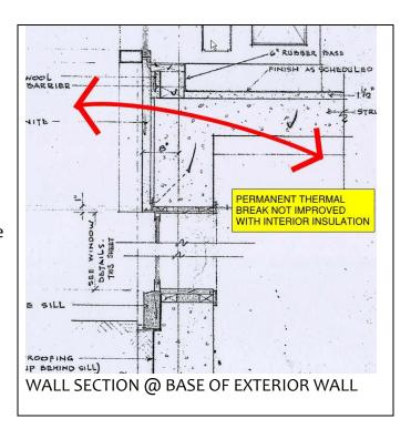
The above noted insulation conditions can only be improved with the implementation of a cavity type wall on the exterior walls. Cavity walls are comprised of an exterior finish, a vented air space, insulation, air barrier and interior wall structure. The existing wall construction can not be retrofitted to a cavity wall without a complete dismantling of the wall and reconstructing a new wall.
