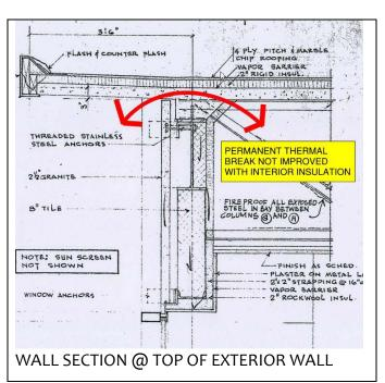
Similar to the sketch above a thermal break at the floor line also occurs and would continue if the exterior walls are left in place.
