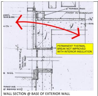
The above noted insulation conditions can only be improved with the implementation of a cavity type wall on the exterior walls. Cavity walls are comprised of an exterior finish, a vented air space, insulation, air barrier and interior wall structure. The existing wall construction cannot be retrofitted to a cavity wall without a complete dismantling of the wall and reconstructing a new wall.
